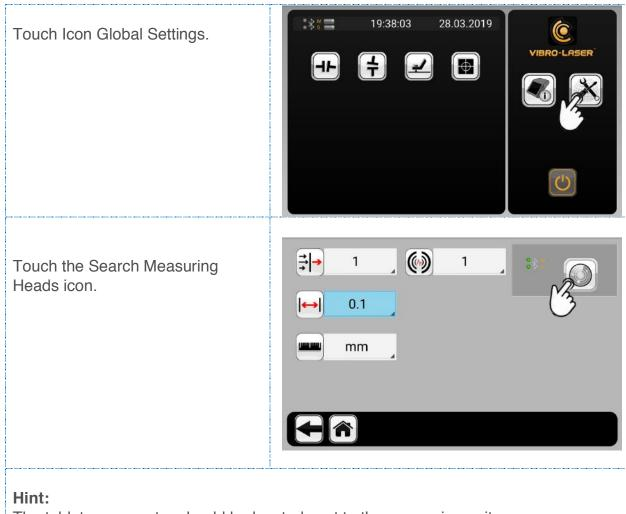
The tablet or computer should be located next to the measuring units.
