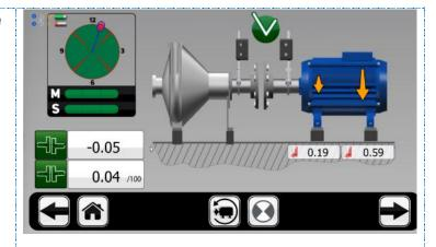
After adjusting the machine in a vertical plane click the live move mode icon.
