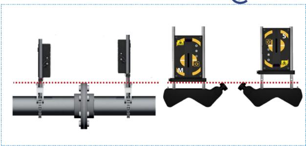
8. We recommend that, in order to improve the measurement accuracy, install the units so that the distance between them is as large as possible, ranging from 0.1 to 10 m.
