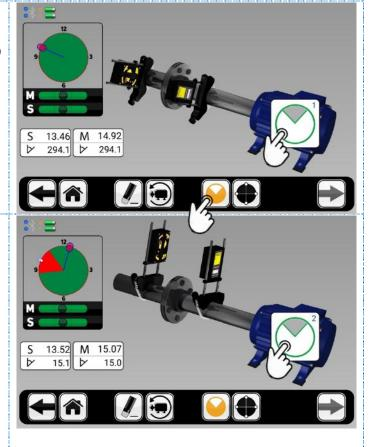
Set the measuring units to the last position and tap the icon Take readings.
