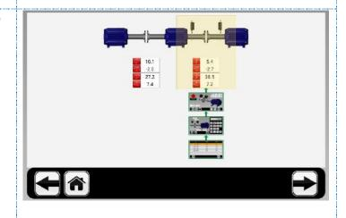
Upon completing the measurements for each coupling, you will then proceed to the current state alignment screen for the entire train.
