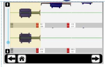
Move forward and you will be shown the shim and move requirements to be made based upon your stationary machine selection.
